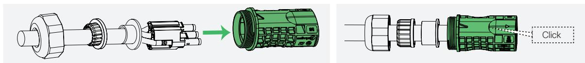
F) Slide the gasket, compression ring, and nut over the cable assembly. Tighten the nut to  $2.5 \pm 0.5$  N·m.
