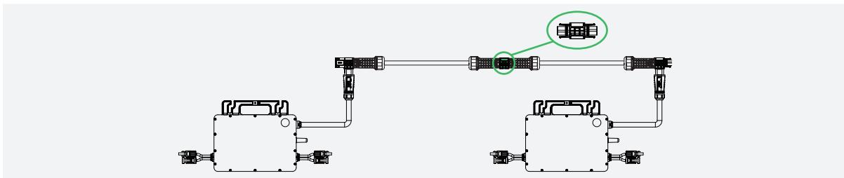
\* To disconnect the Flex-S3 Extension Connector from the AC Trunk, you must use a Flex-S3 Disconnect Tool. (See "[7.1 Removing the Microinverter](#)".)
