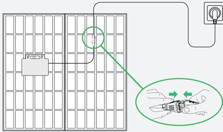
**Procedure****Step 1 Attach the microinverter to the PV racking**
