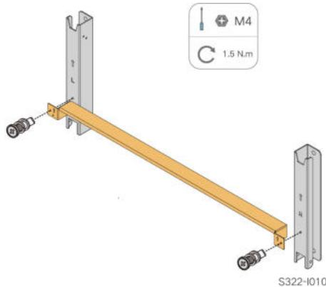
**Step 2** Level the assembled mounting-bracket by using the level, and mark the positions for drilling holes on the PV bracket. Drill the holes by using a electric drill.
