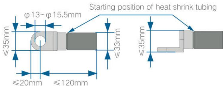
**Figure 5-5** Specifications of the Crimped OT/DT Terminal
