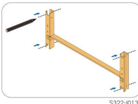
**Step 3** Insert the expansion bolts into the holes and secure them with a rubber hammer. Fasten the nut with a wrench to expand the bolt. Remove the nut, spring washer, and flat washer, and store them properly.
