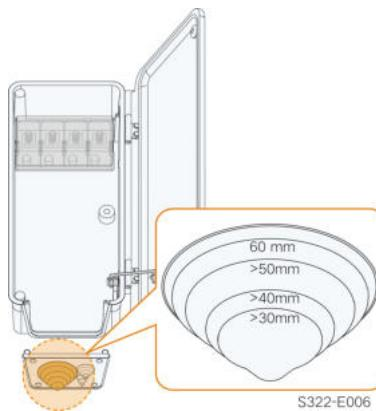
**Step 5** Lead the cable with the protective layer stripped through the sealing ring and secure screws on the bottom sealing plate.
