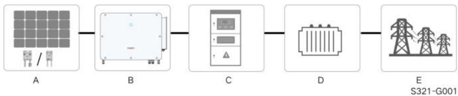
**Figure 2-1** Inverter Application in PV Power System
