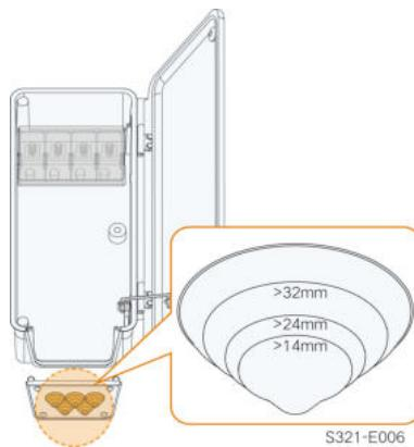
**Step 5** Lead the cable through the sealing ring and secure the screws on the bottom sealing plate.
