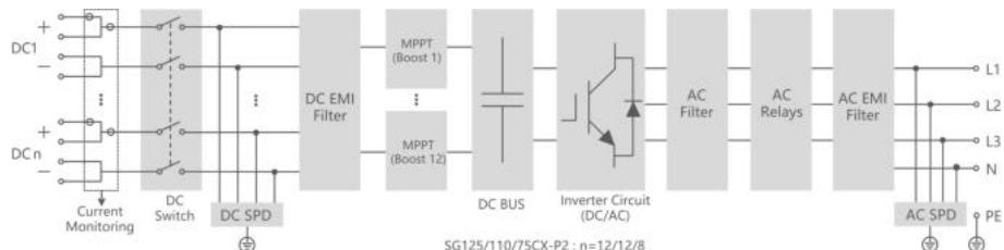
Figure 2-4 Circuit Diagram
