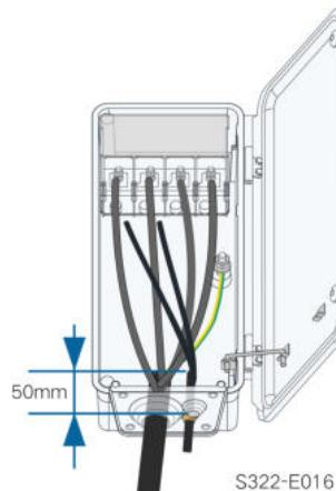
**Step 4** Place the OT terminals of power cable for tracking system on the OT/DT terminals of the AC cable, and secure them.
