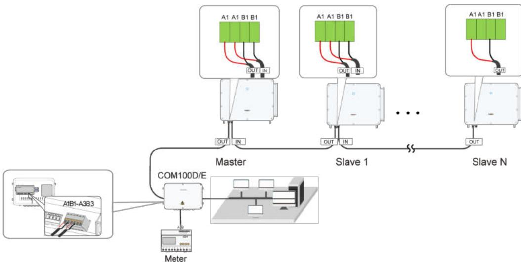
**Figure 5-6 Multi-inverter Communication System [RS485\_1 interface (terminal block)]**
