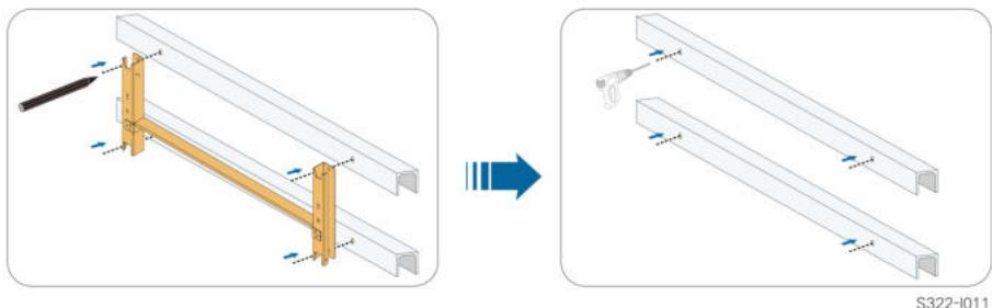
**Step 3** Secure the mounting-bracket with bolts.
