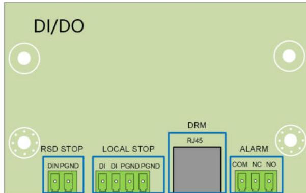
**DO terminal (fault output dry contact)**
