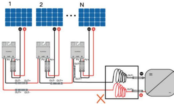
**Step 4** Connect the PV connectors to corresponding terminals until there is an audible click.
