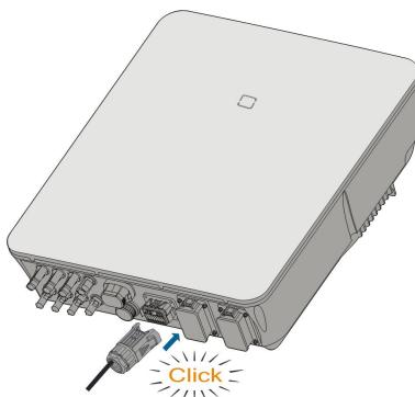
**Step 3** Pull cables outwards to confirm whether they are fastened firmly.
