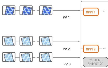
For SH10RT/SH10RT-20, if two PV strings are paralleled externally, the paralleled strings can be connected to PV2 or PV3 only, and the other one cannot be used to connect other PV strings.
