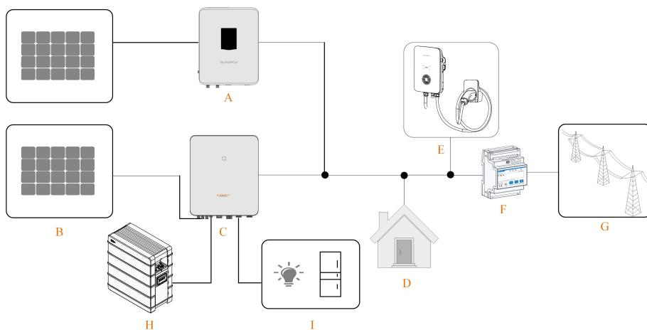
**Figure 2-8** Retrofitted PV Storage and EV-Charger System
