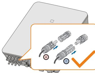
**Step 2** Check for polarity correctness.
