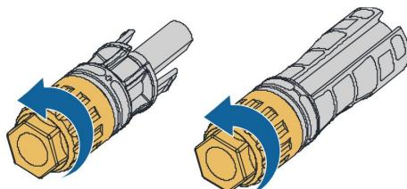
**Step 3** Lead the stripped cable through the swivel nut and insert it into the insulation sleeve till the end.
