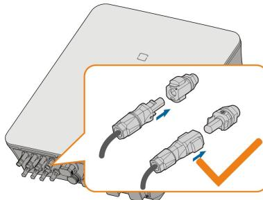
**Step 2** Ensure that the connectors are securely in place.
