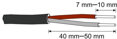
**Step 5** Plug the wires into the **RS485** terminal according the labels on the bottom of the inverter.
