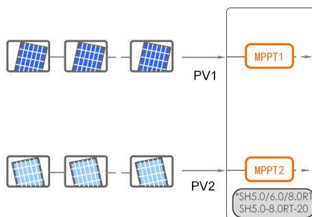
For SH10RT/SH10RT-20, each pair of PV terminals is corresponding to an independent PV string. PV input PV1 connect to MPPT1 and PV2, PV3 connect to MPPT2. For the best use of PV power, PV2 and PV3 should be the same in PV string structure, including the type, number, tilt, and orientation of the PV modules.
