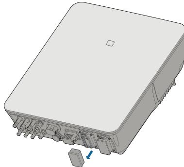
**Step 4** Align the Backup connector and the **BACK-UP** terminal and mate them together by hand until a “Click” is heard or felt.
