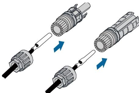
**Step 4** Screw the swivel nut of the connector and gently pull the cable backward to ensure a firm connection.
