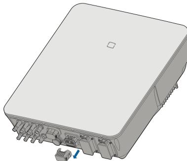
**Step 2** Insert the COM connector into **COM** terminal on the bottom of the inverter until there is an audible click.
