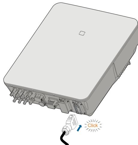
**Step 4 (Optional)** Insert the block into AC connector, as shown in the figure below.
