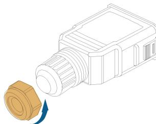
**Step 2 (Optional)** Remove the inner sealing ring if the cable diameter is between 19 mm ~ 25 mm. Otherwise skip this step.
