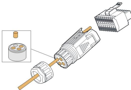
**Step 4** Remove the cable jacket by 7 mm–10 mm.
