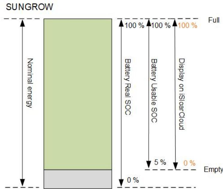
The SOC limits of Li-ion batteries can be modified via the iSolarCloud App by qualified personnel.
