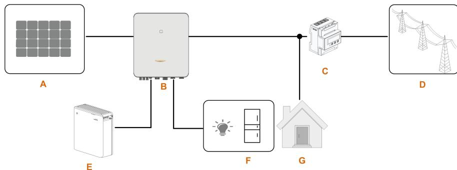
**Figure 2-3 PV Energy Storage System (PV ESS)**
