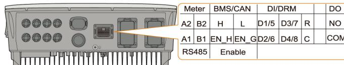
**Figure 6-2** The label description of COM terminal
