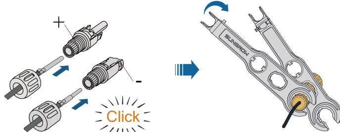
**Step 4** Check for polarity correctness.
