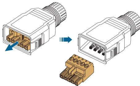
**Step 4** Thread the AC cable of appropriate length through the swivel nut and the housing.
