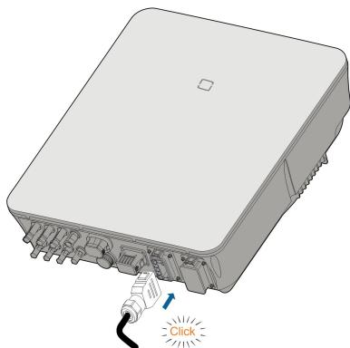
**Step 5** Pull all the lines outward to check whether they are firmly installed.
