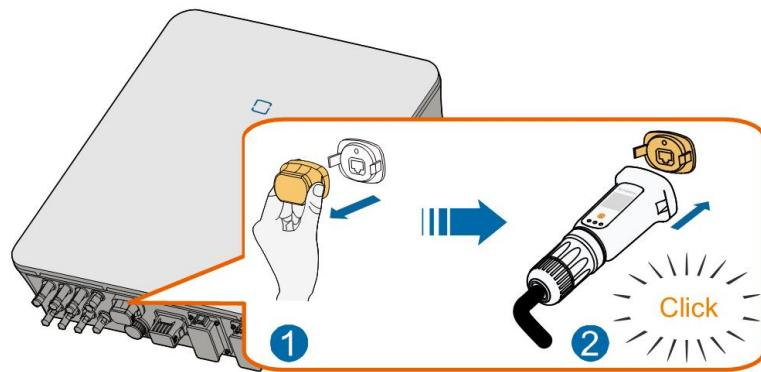
**Step 7** Slightly shake it by hand to determine whether it is installed firmly.
