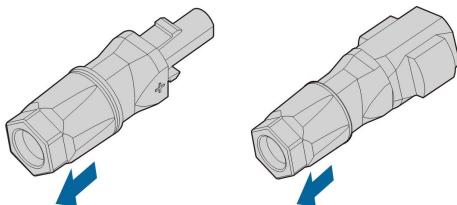
**Step 3** Insert the stripped cable into the cable gland up to the stop. The stranded wire can be seen inside the spring. Press the spring down until it audibly snaps into place.
