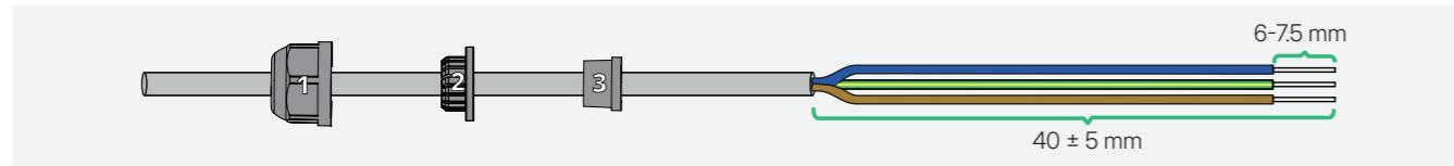
d. Insert the exposed conductors into the terminal pins, crimp them, and push the crimped ends into the connector body.
